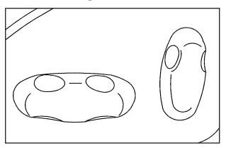
If the seats have power reclining seatbacks, use the vertical power seat control located on the outboard side of each seat.
